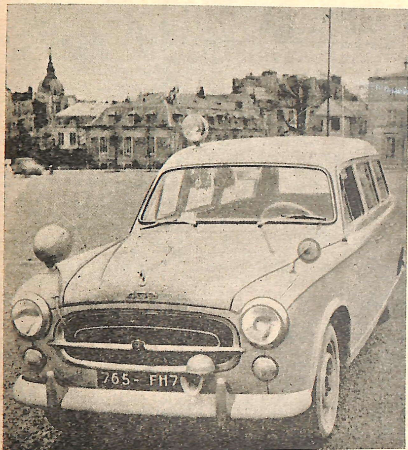
Car fitted with a Traffipax. There is a camera on the right and left hand side of the car. Fitted on the right front side is an instrument for showing date and time of the offence and the speed of the patrol car.
